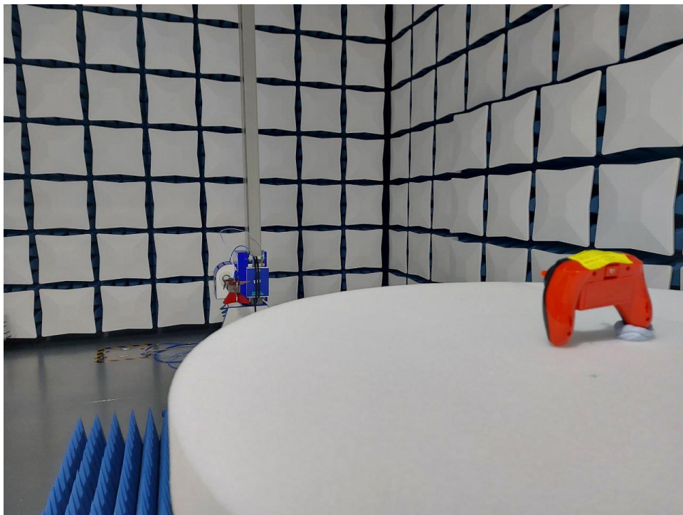
Set-up for Radiated Emission (1GHz above)
