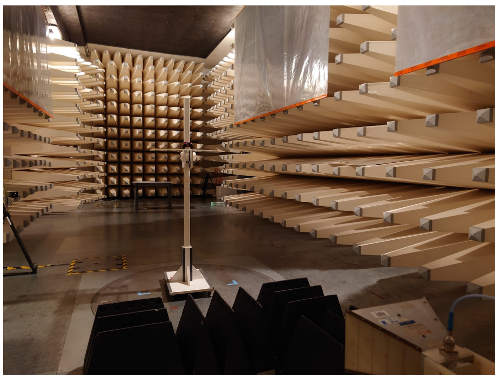
Set-up for Radiated Emission (1GHz above)
