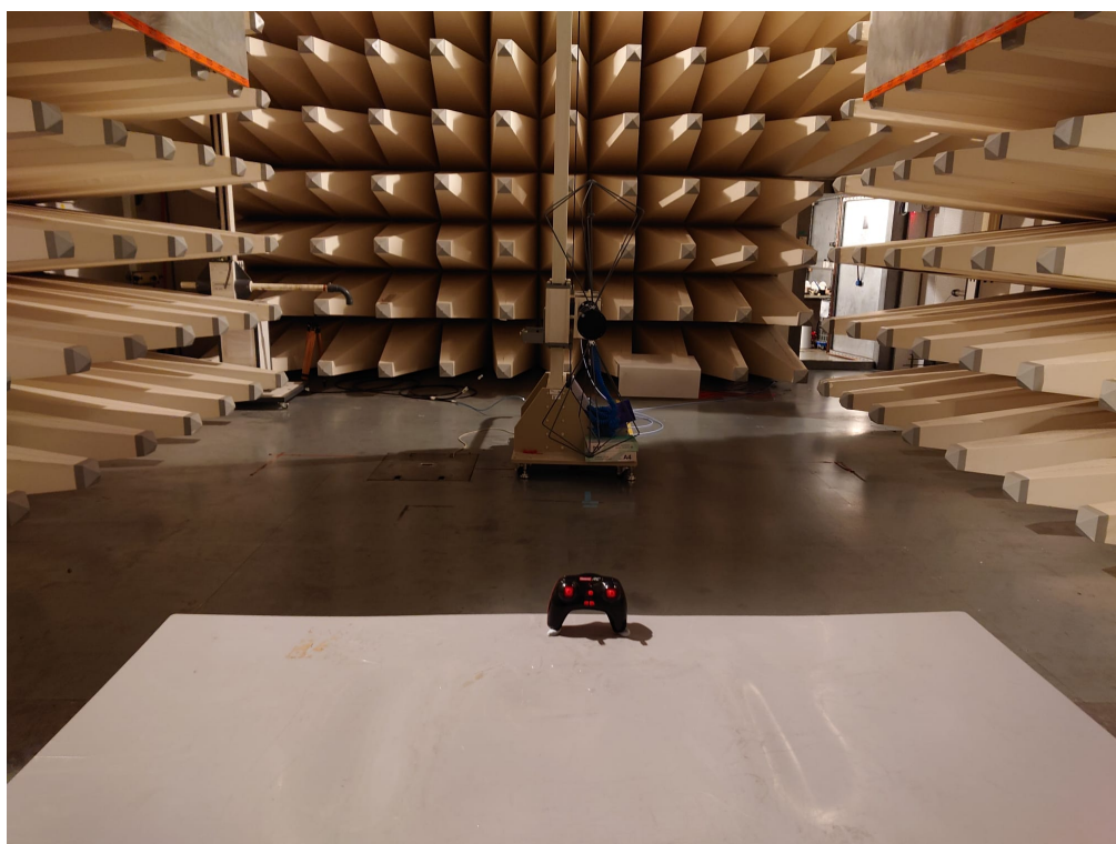
Set-up for Radiated Emission (30-200MHz)
