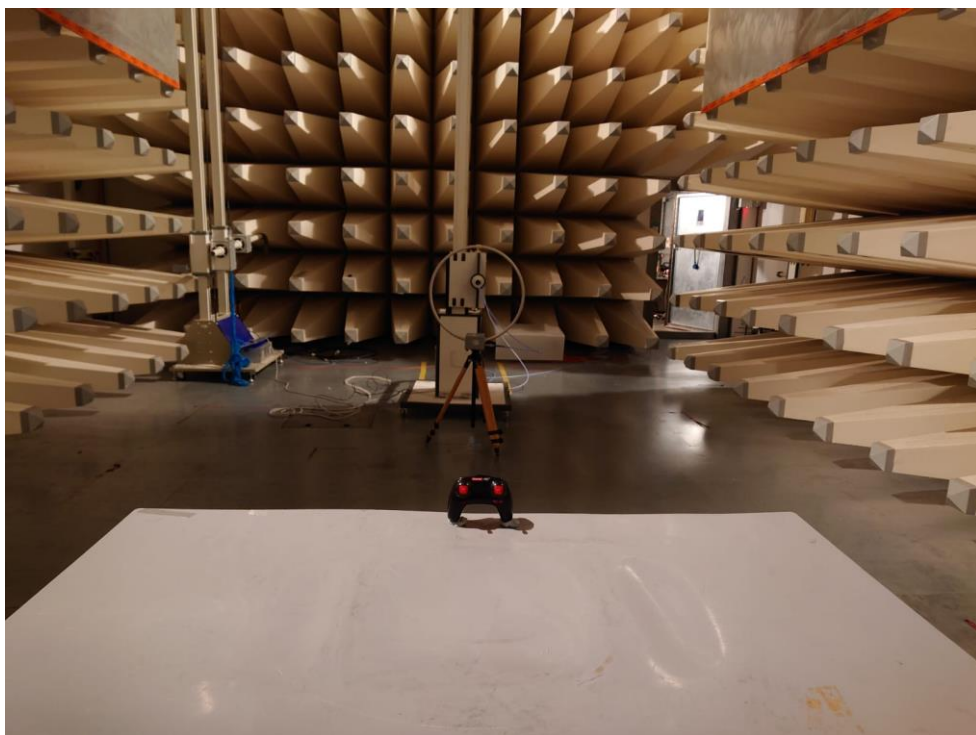
Set-up for Radiated Emission (9k-30MHz)
