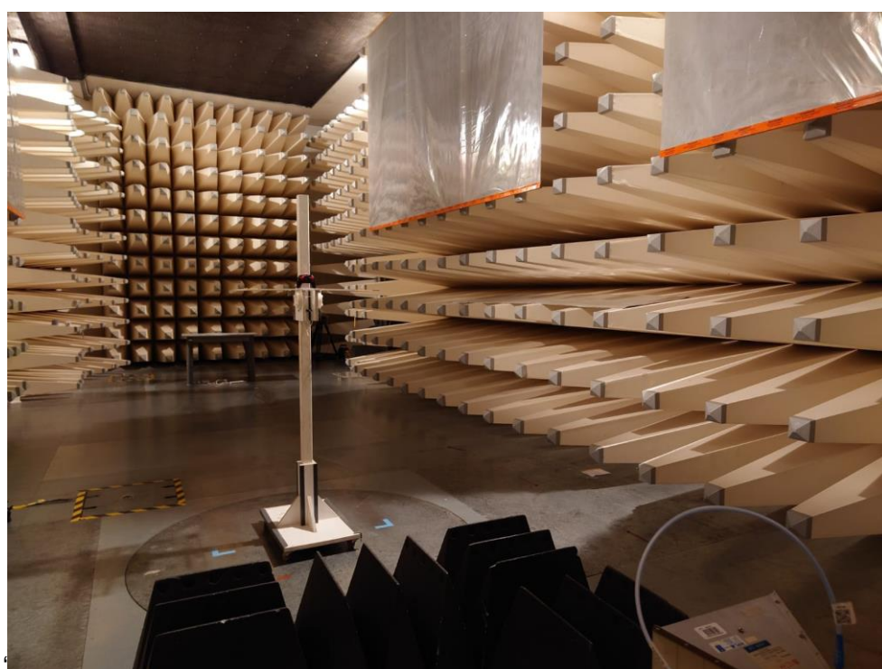
Set-up for Radiated Emission (1GHz above)
