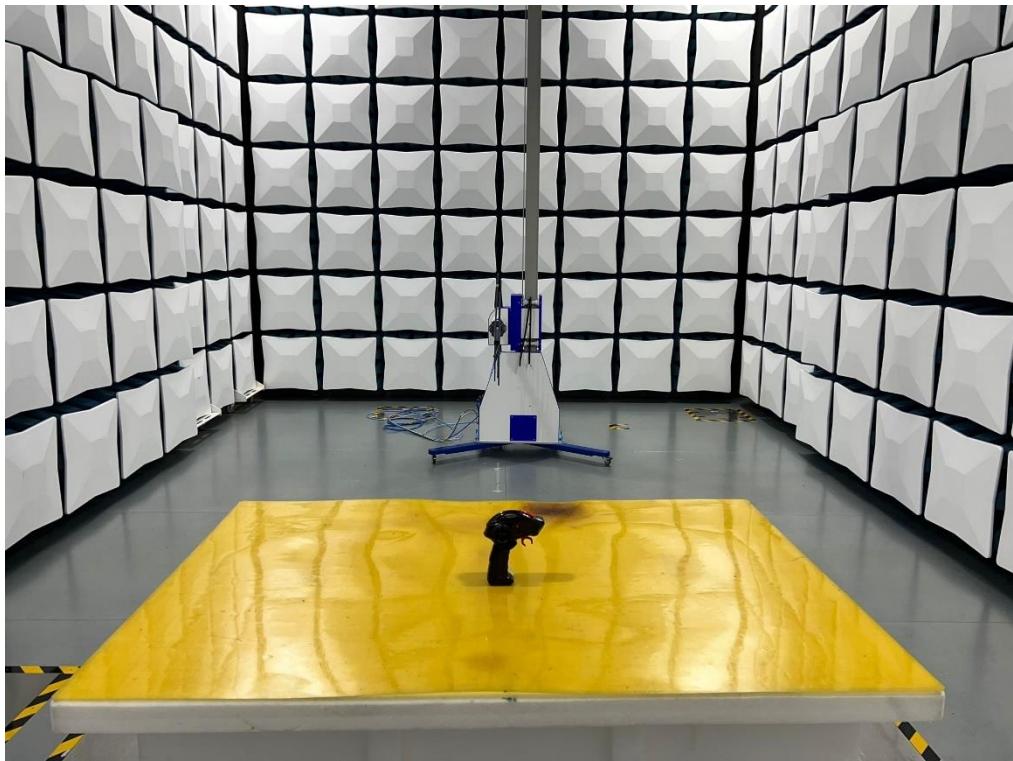
Set-up for Radiated Emission (200M-1GHz)
