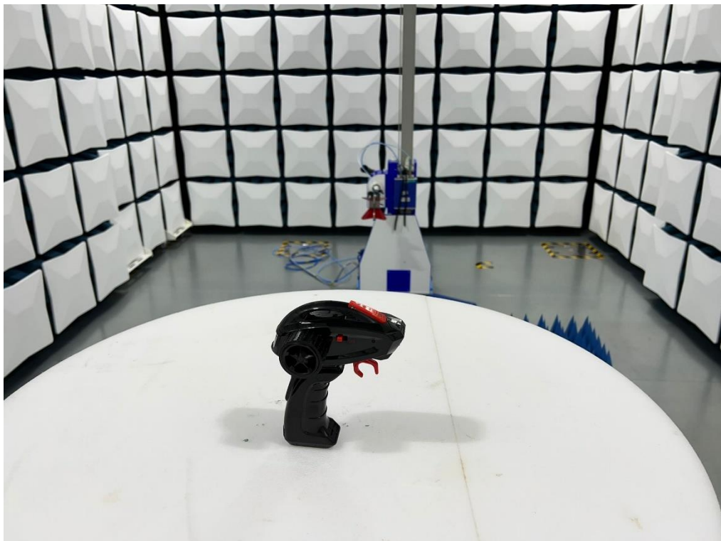
Set-up for Radiated Emission (1GHz above)
