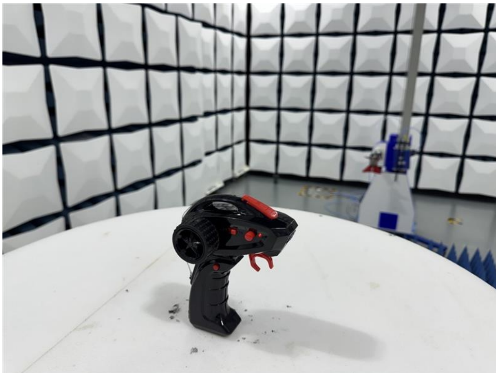
Set-up for Radiated Emission (1GHz above)
