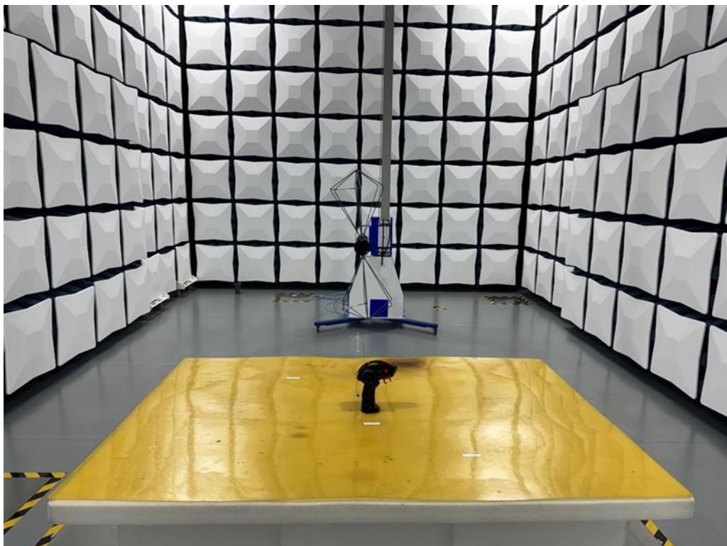
Set-up for Radiated Emission (30MHz-200MHz)
