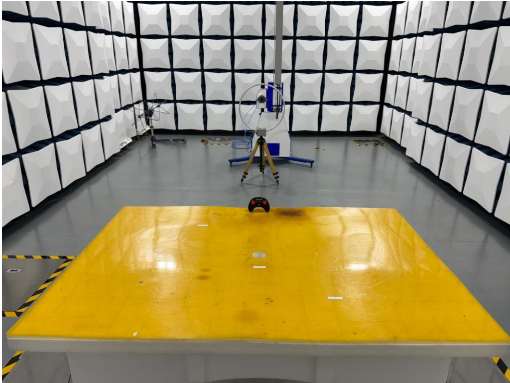
Set-up for Radiated Emission (9kHz-30MHz)
