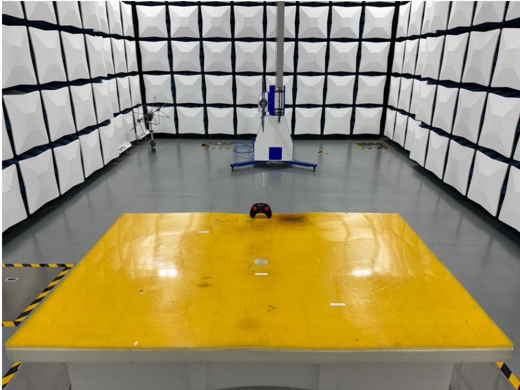
Set-up for Radiated Emission (200MHz-1000MHz)
