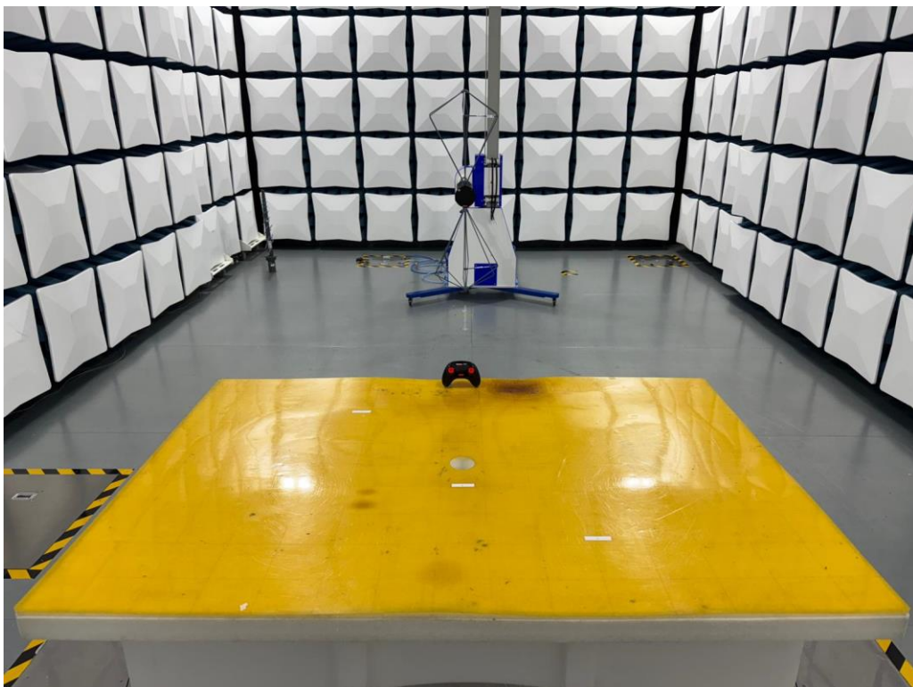
Set-up for Radiated Emission (30MHz-200MHz)
