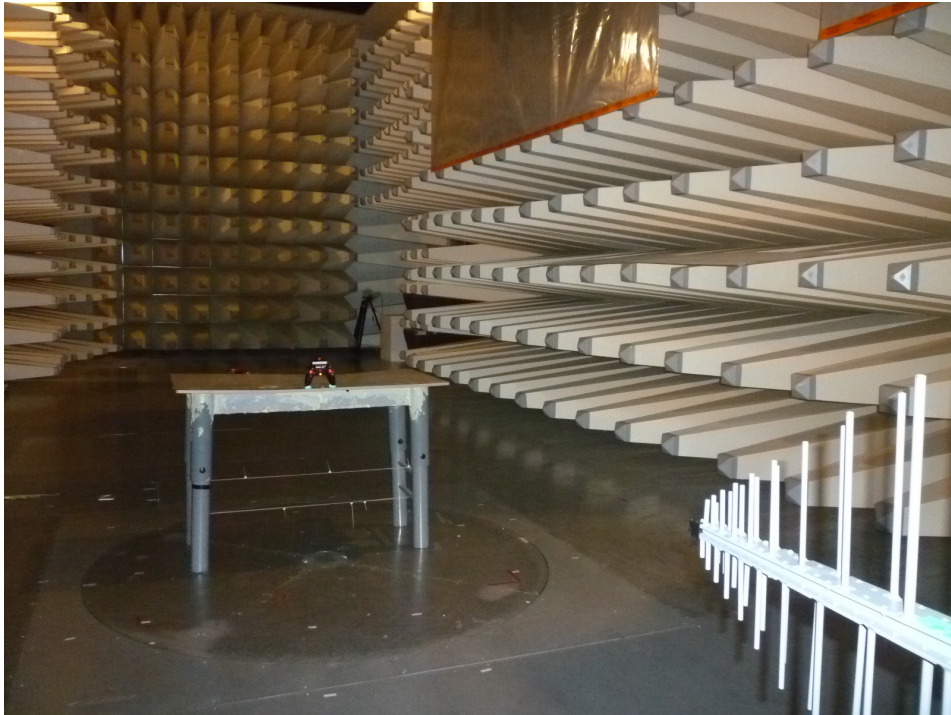
Setup for radiated emission
