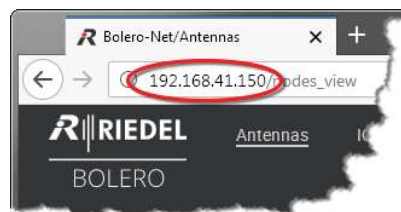
Figure 34: Web interface of the Antenna
