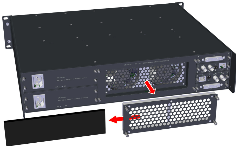
figure 19: replacing rear filter
