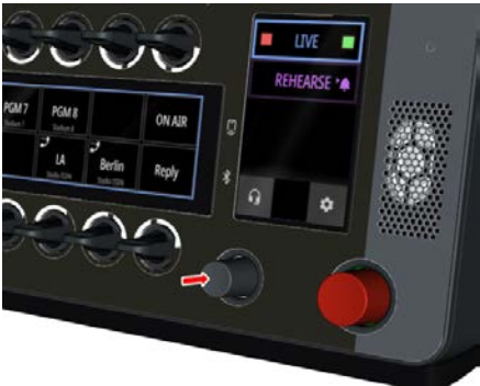
figure 16: microphone muting (DSP-1216HL)
