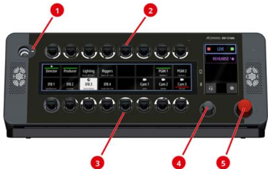
figure 10: DSP-1216HL (front status LED positions)
