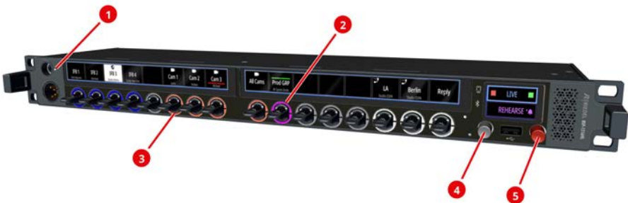
figure 20: front status LED positions (RSP-1216HL)
