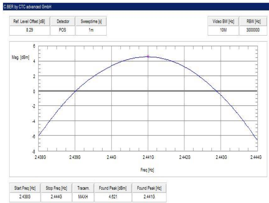
Plot 8: middle channel – 2441 MHz, 8 DPSK modulation
