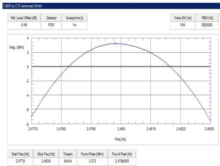
Plot 3: highest channel – 2480 MHz, GFSK modulation
