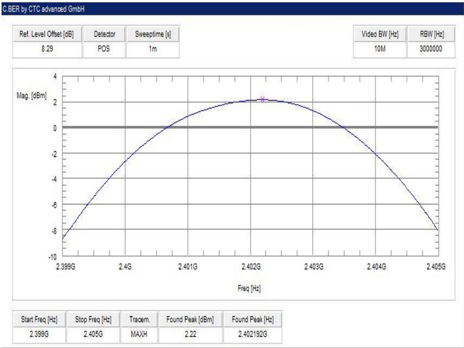
Plot 1: lowest channel – 2402 MHz, GFSK modulation
