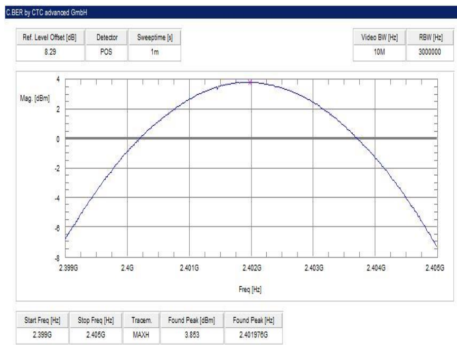
Plot 7: lowest channel – 2402 MHz, 8 DPSK modulation
