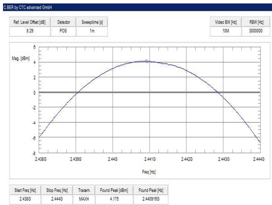
Plot 5: middle channel – 2441 MHz, Pi / DQPSK modulation
