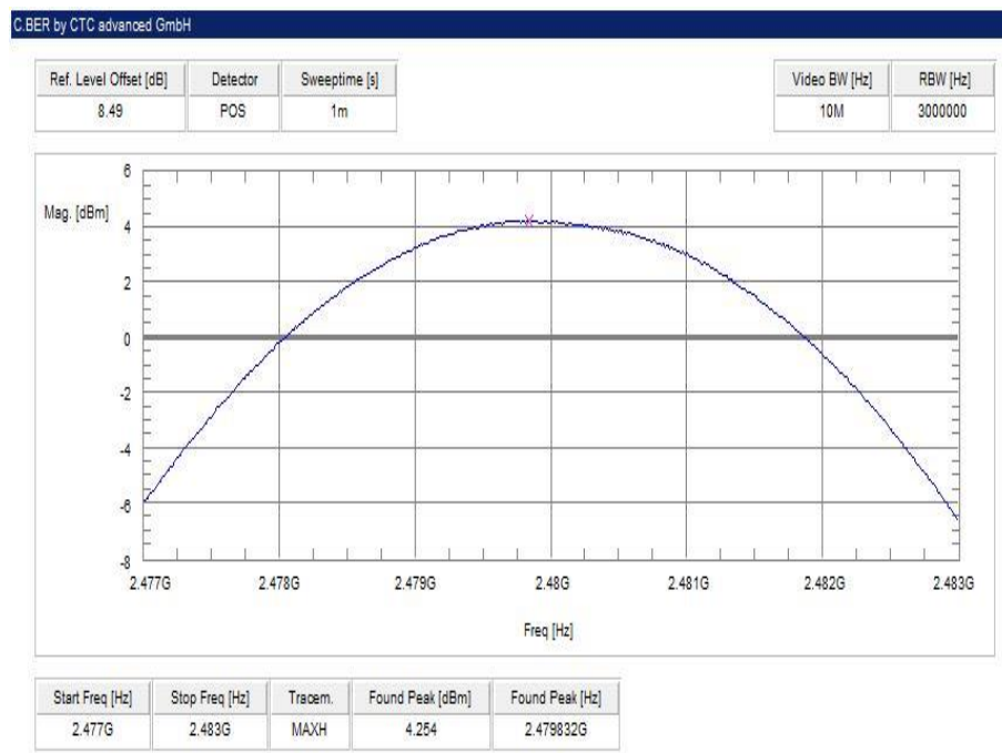
Plot 6: highest channel – 2480 MHz, Pi / DQPSK modulation
