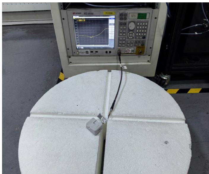
Free Space Impedance Setup (USB receiver)
