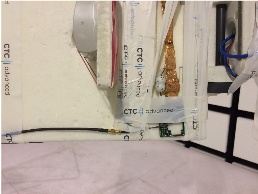
Photo 3: RSE set-up (>1GHz)
