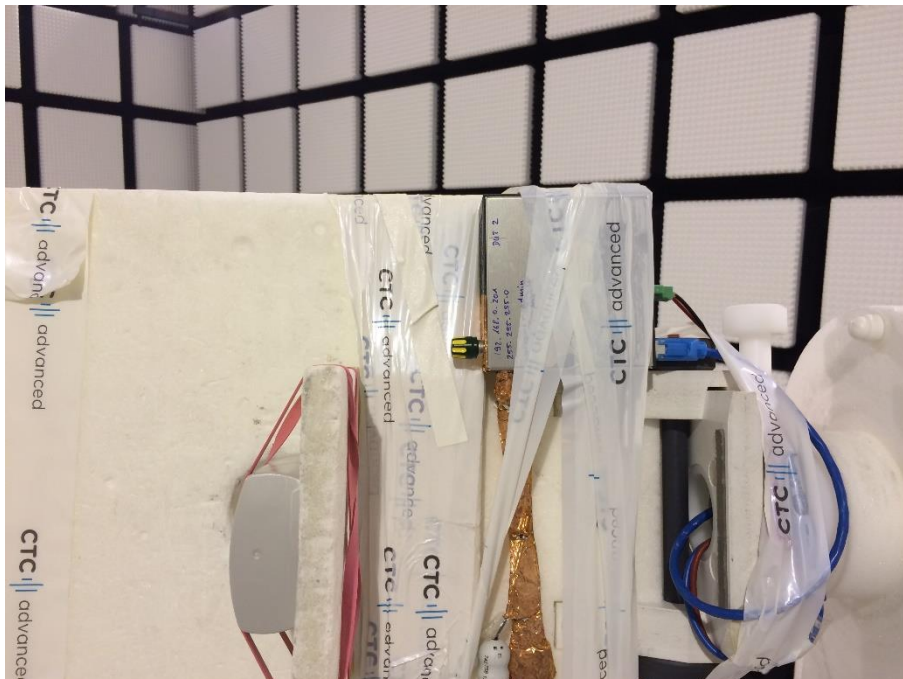
Photo 4: RSE set-up (>1GHz)
