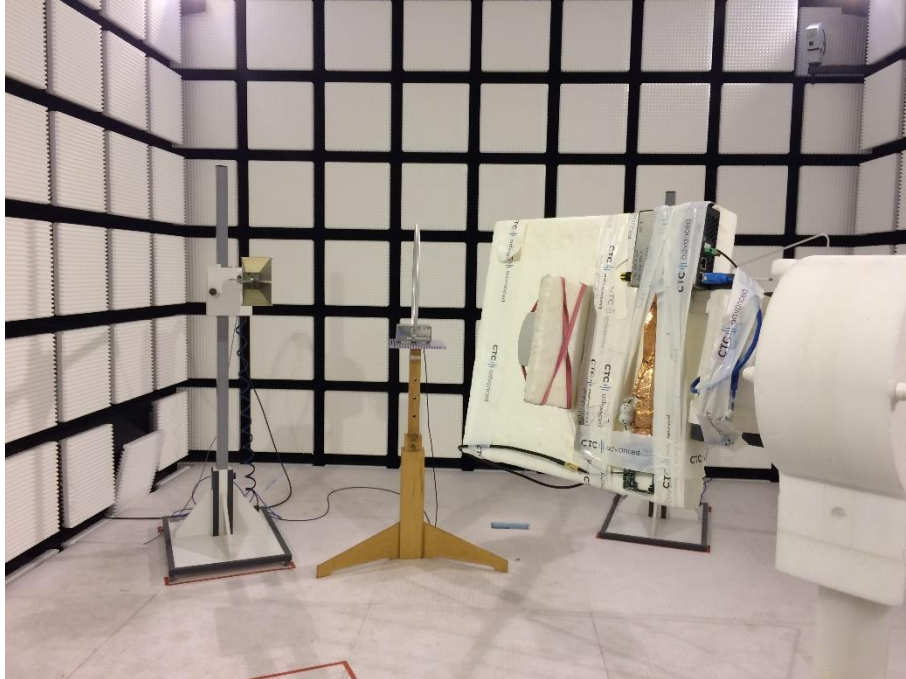
Photo 5: RSE set-up (>1GHz)
