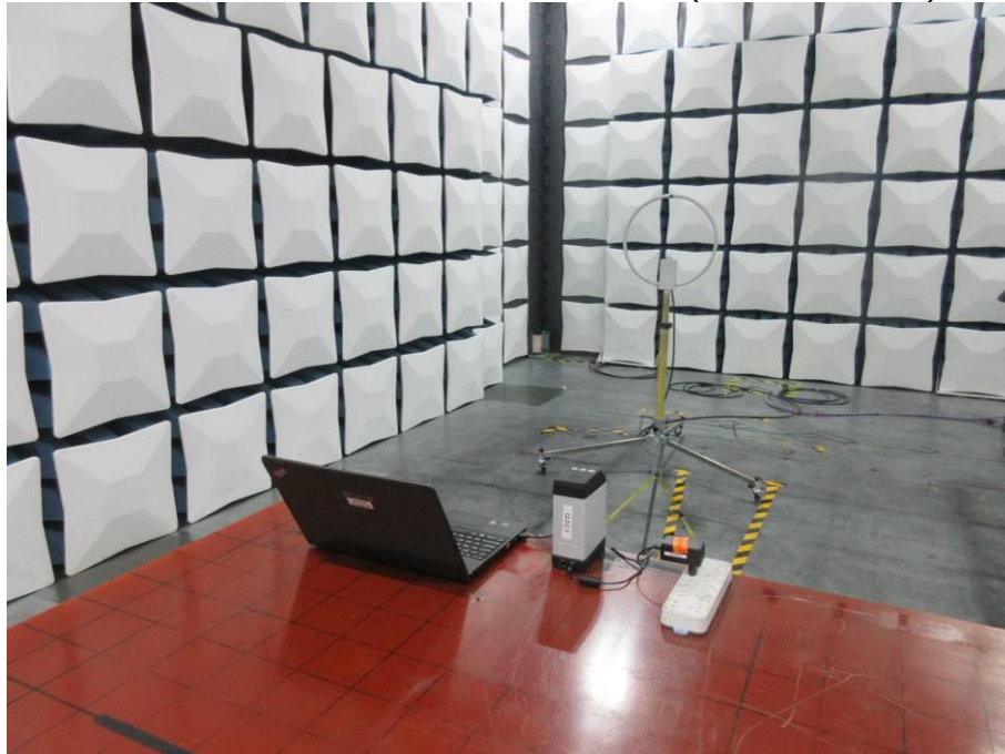
RADIATED RF MEASUREMENT SETUP (9KHz ~ 30 MHz)
