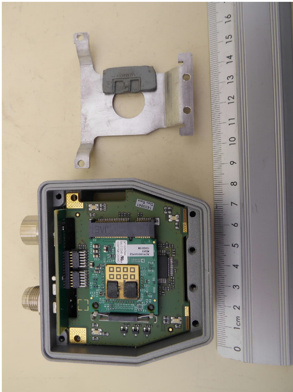
NEARFI 2000 B, internal view 2, shielding removed
