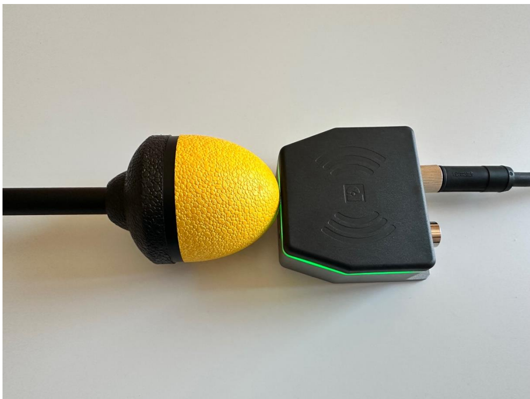
Photo : 17 – 10 MHz & 60 GHz field probe measurements – exemplary
