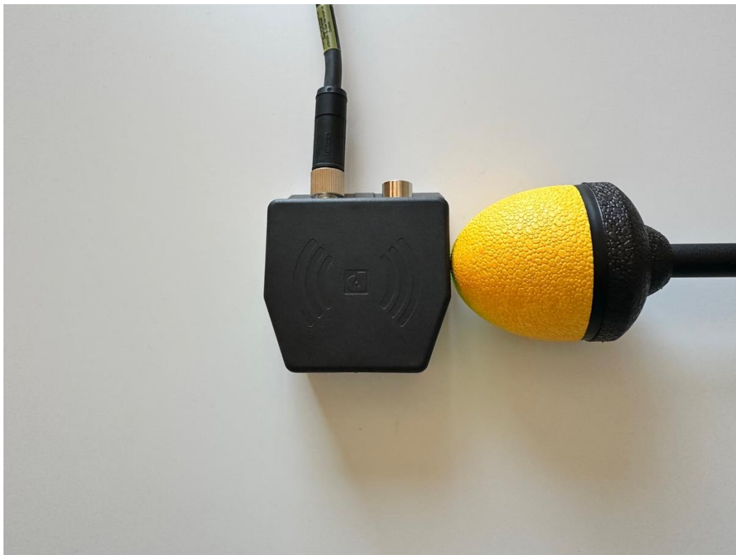
Photo : 16 – 10 MHz & 60 GHz field probe measurements - exemplary
