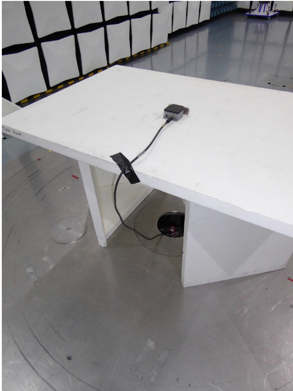
Test setup semi anechoic chamber (position 3)
