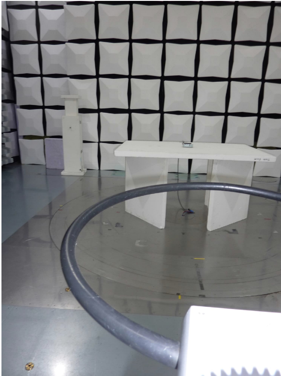
Test setup semi anechoic chamber <30 MHz
