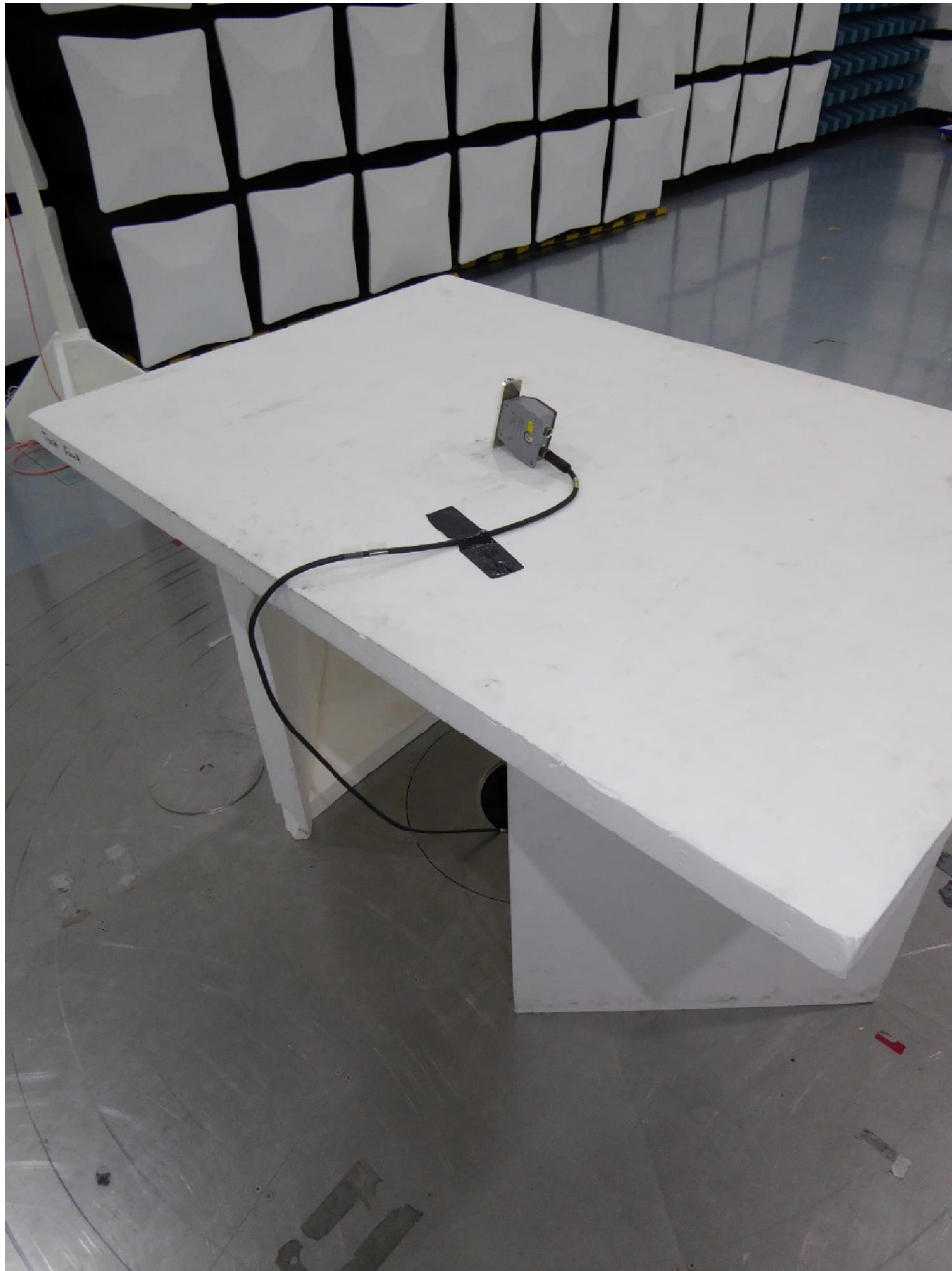
Test setup semi anechoic chamber (position 2)
