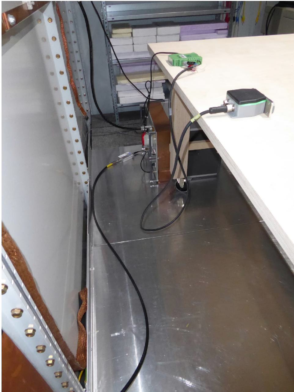
Test AC power line conducted emissions
