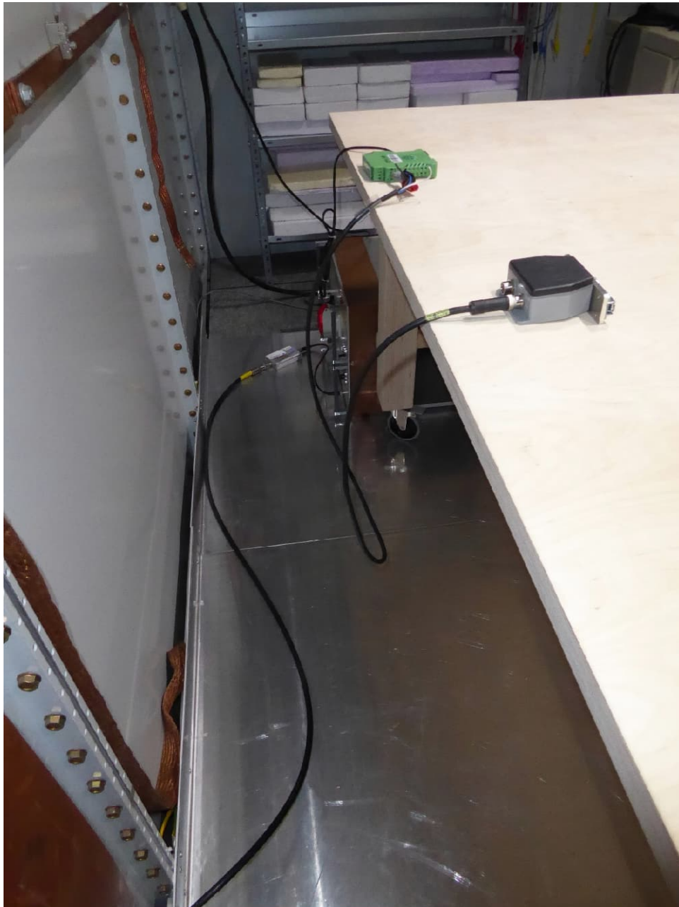
Test AC power line conducted emissions
