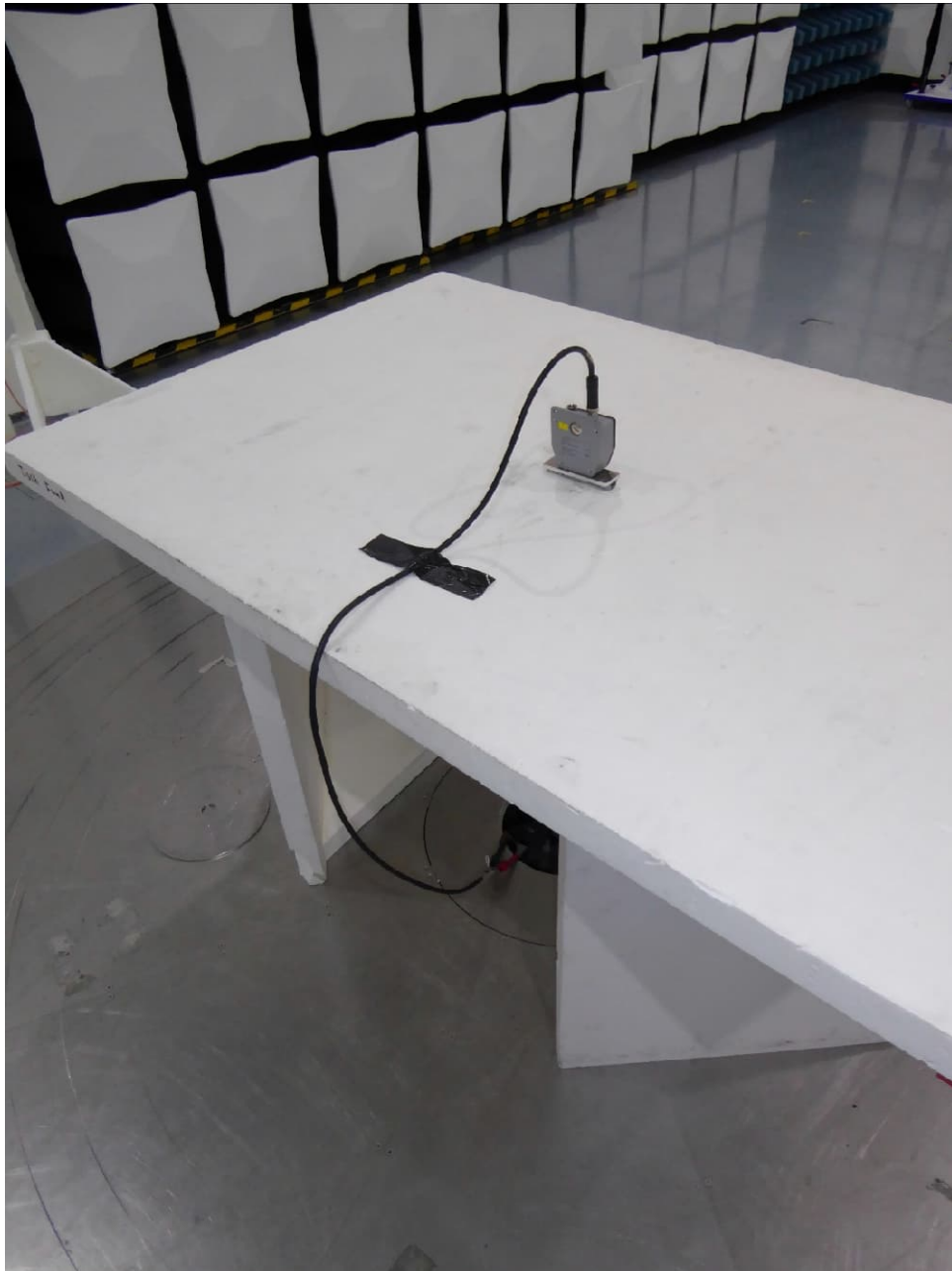
Test setup semi anechoic chamber (position 1)
