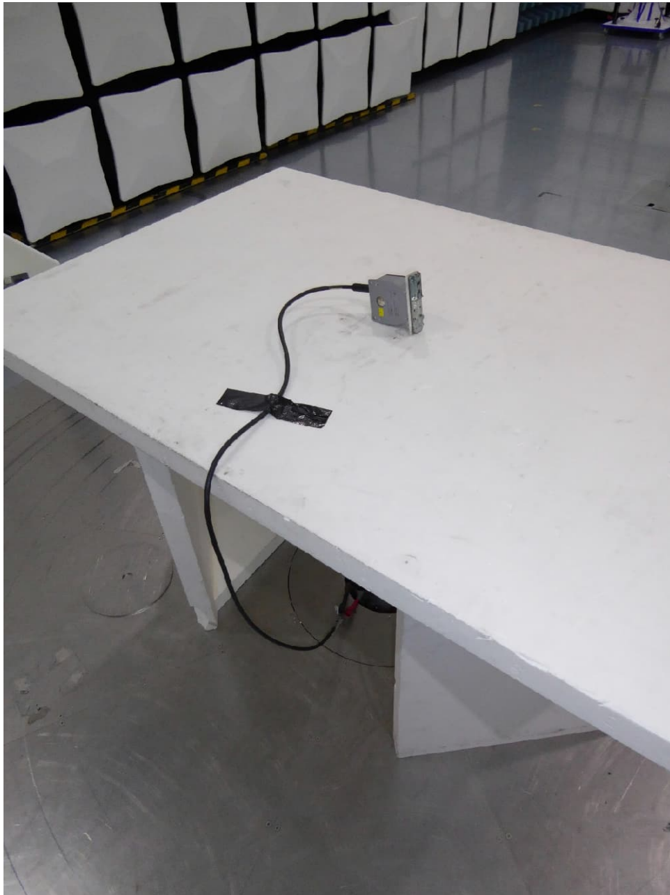
Test setup semi anechoic chamber (position 2)
