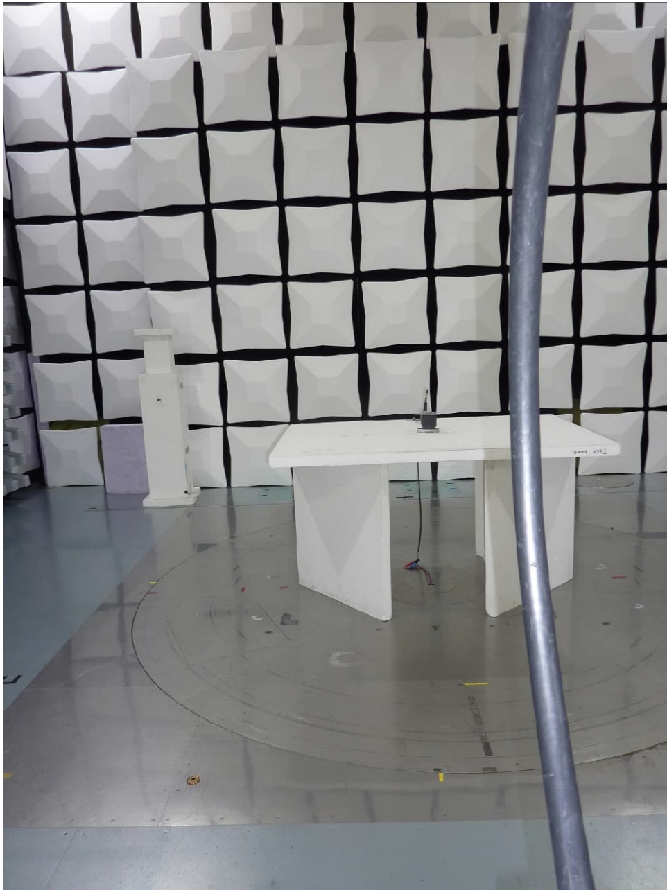
Test setup semi anechoic chamber <30 MHz
