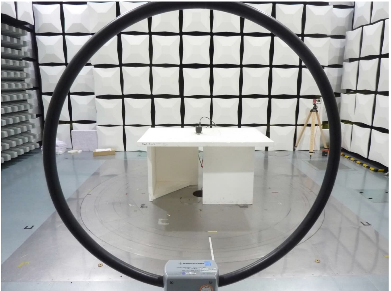
Test setup semi anechoic chamber <30 MHz
