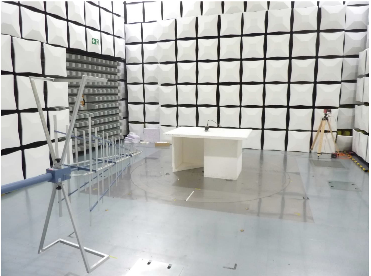
Test setup semi anechoic chamber <1 GHz
