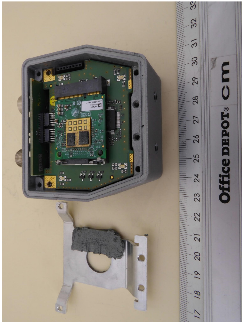
NEARFI PD 2A ETH B, internal view 2, shielding removed
