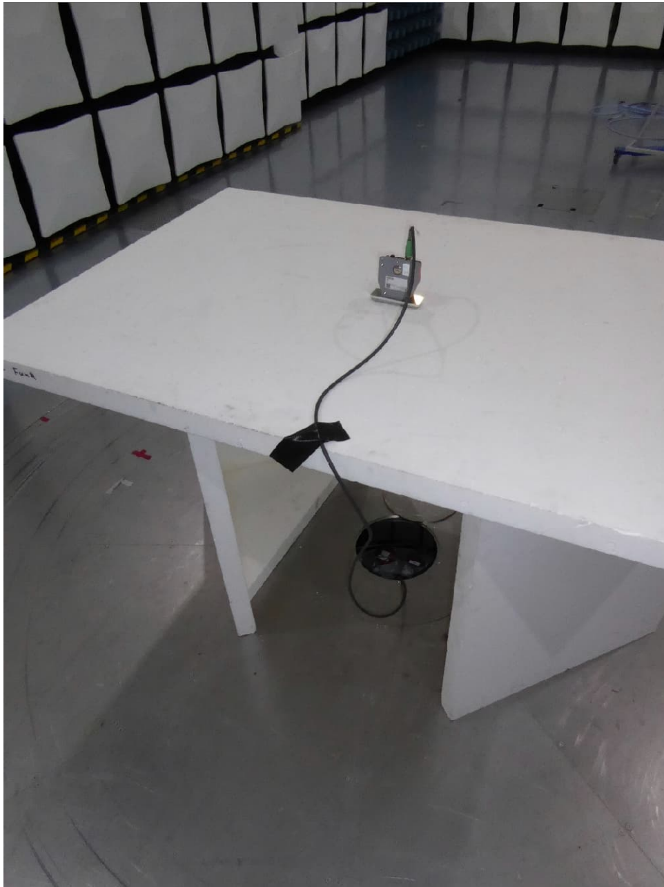
Test setup semi anechoic chamber (position 1)
