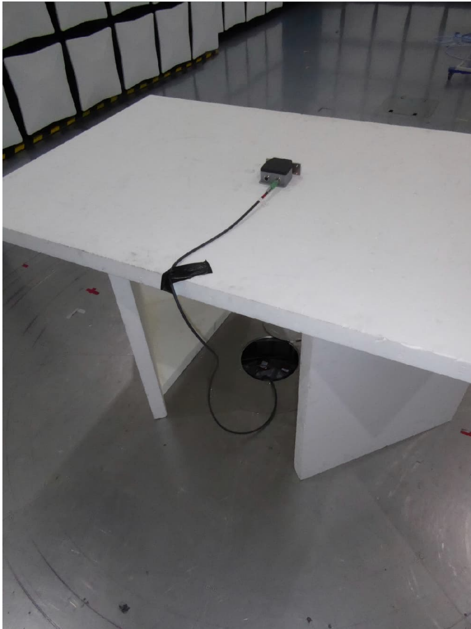
Test setup semi anechoic chamber (position 3)
