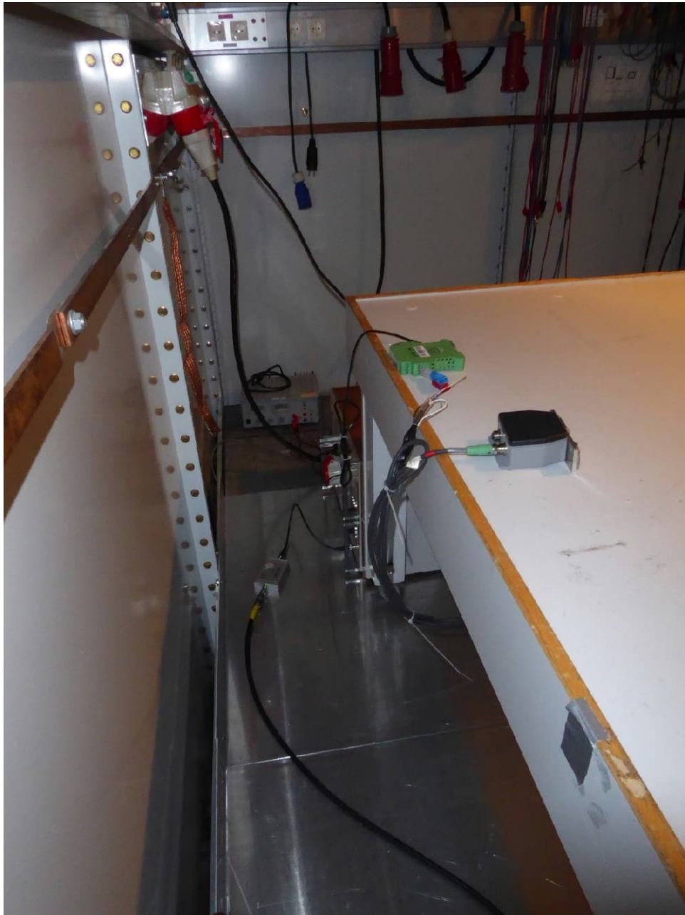
Test AC power line conducted emissions
