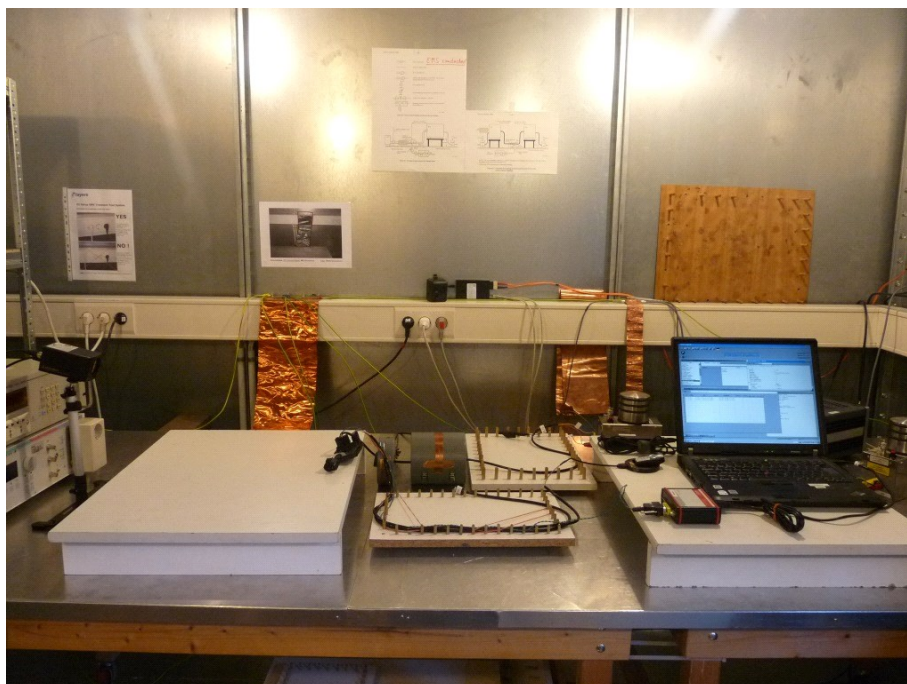
Picture 7 : setup for the test "RF-common mode"
