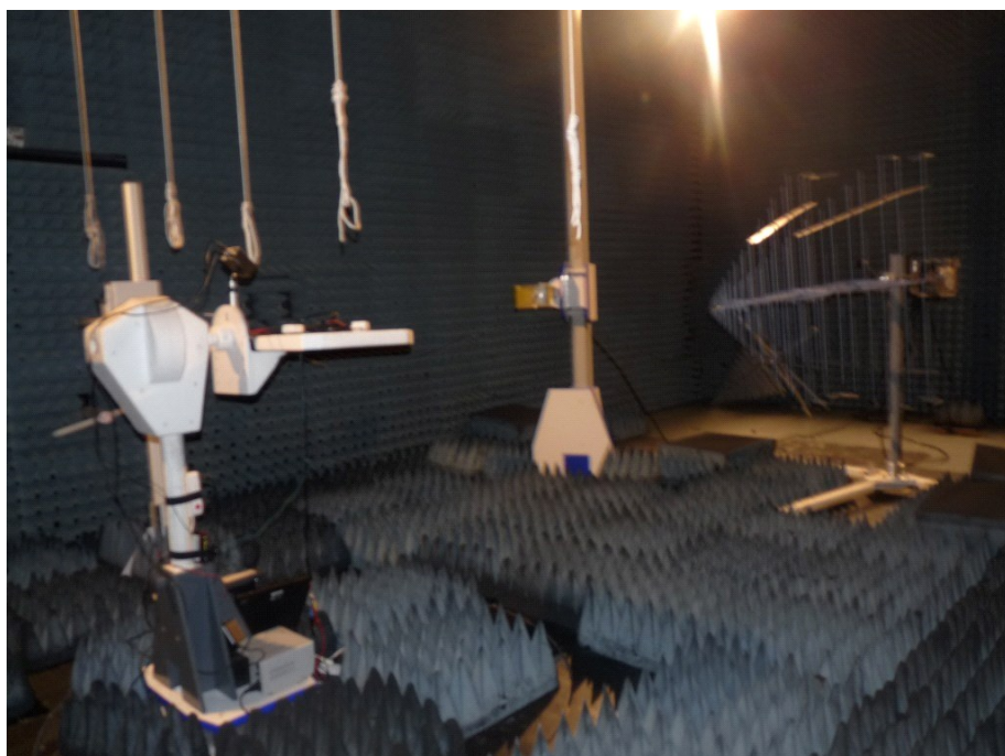
Picture 6 : setup for the test "RF-electromagnetic field"
