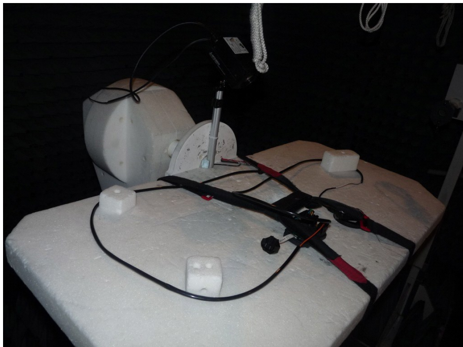
Picture 5 : setup for the test "RF-electromagnetic field", detailed view
