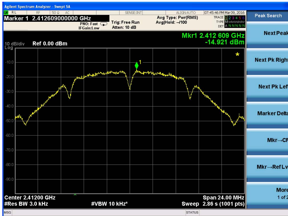
Power spectral density plot on channel 6
