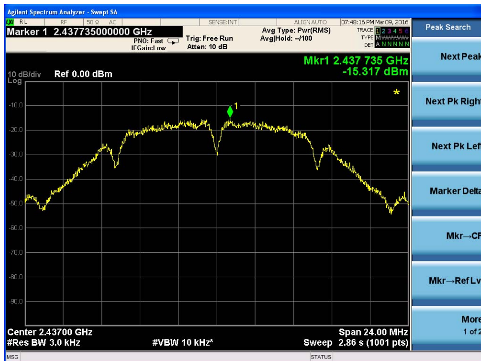
Power spectral density plot on channel 6
