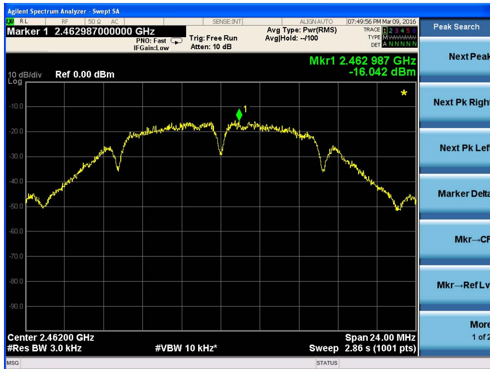
Power spectral density plot on channel 1
