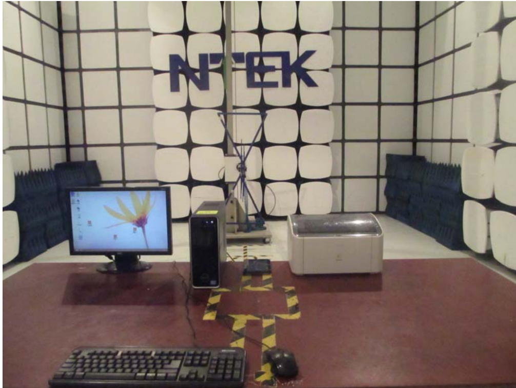
Radiated Measurement Photos
