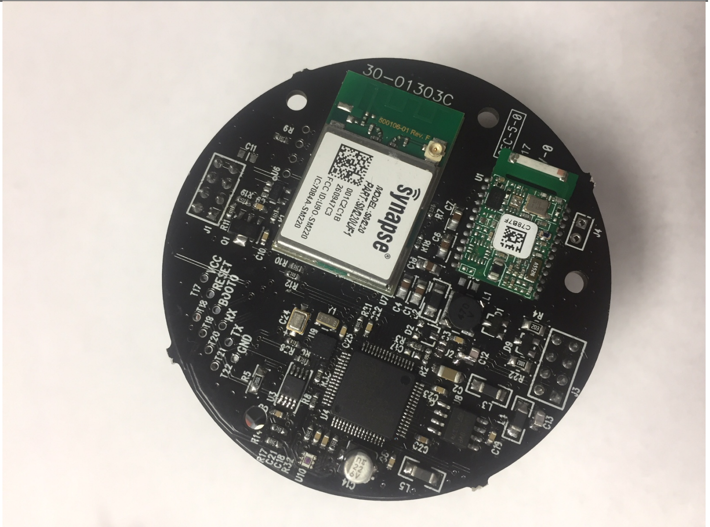
Board 2 Top; control board
