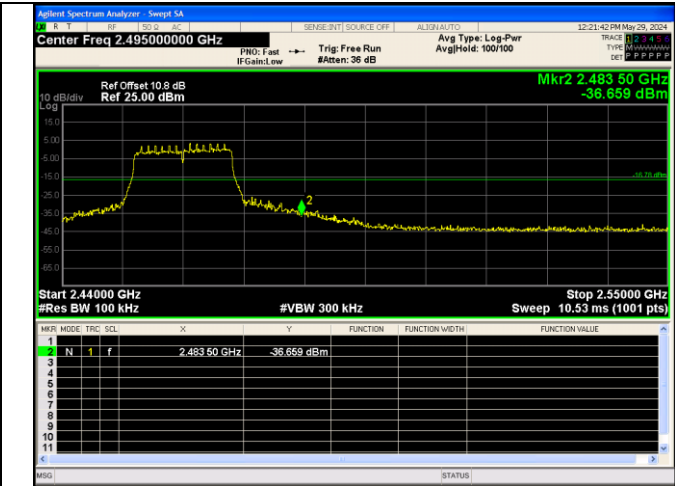
Out Of Band Emission IEEE 802.11n Channel 11 20MHz Antenna 0
