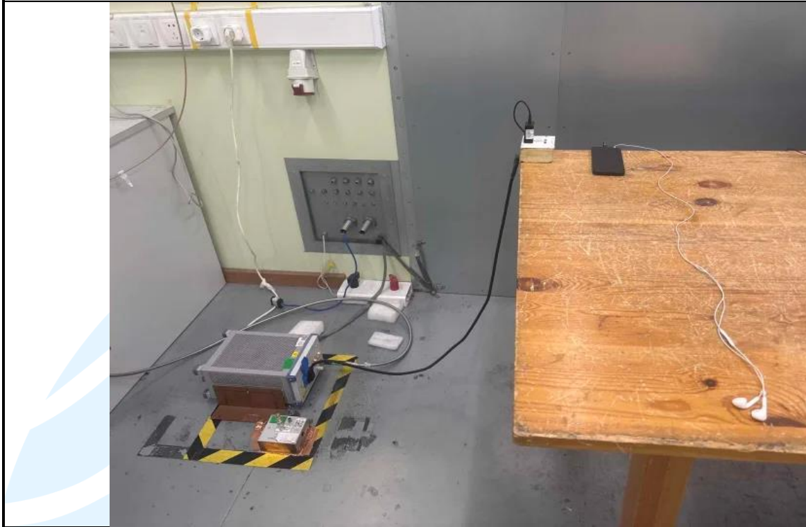
Conducted Emission Test Setup
