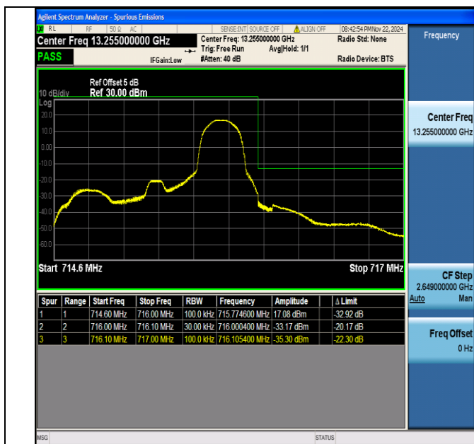
Band12 1.4MHz 64QAM 23173 1RB#5
