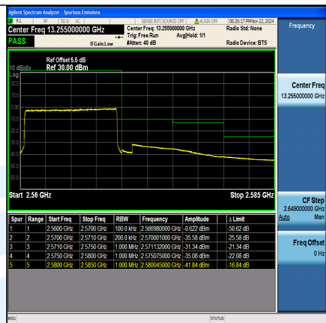
Band7 10MHz 64QAM 21400 50RB#0
