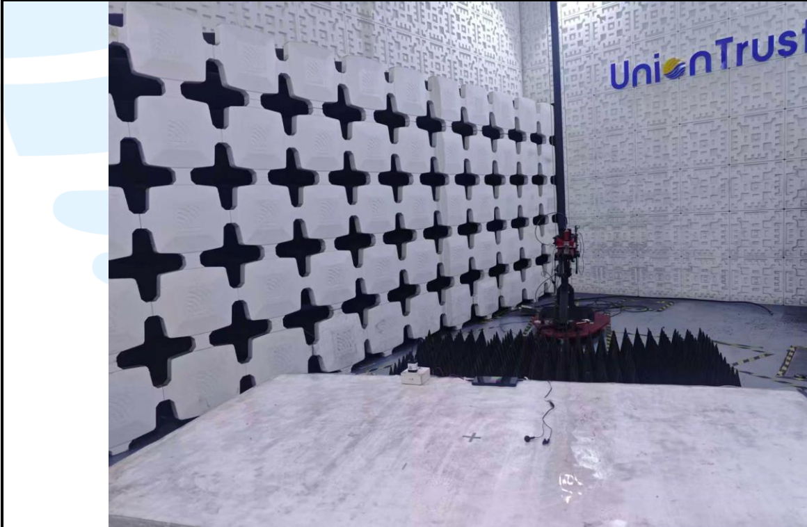
Radiated emission Test Setup-2 (Above 1 GHz)
