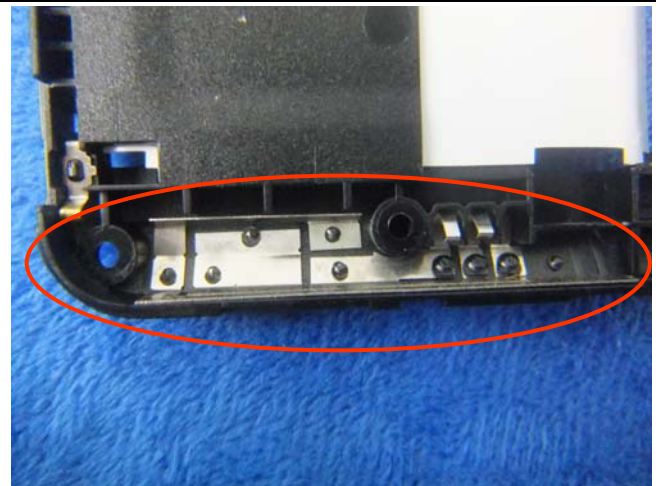
GSM/PCS/UMTS-FDD Antenna View
