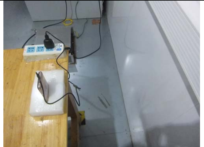
Conducted Emissions Test Setup Side View
