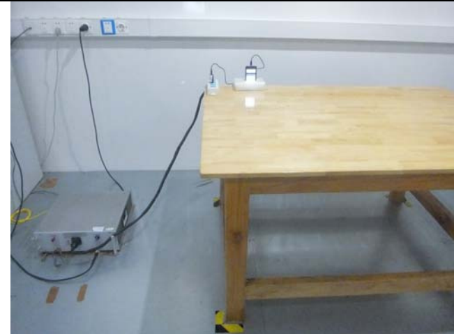
Conducted Emissions Test Setup Front View
