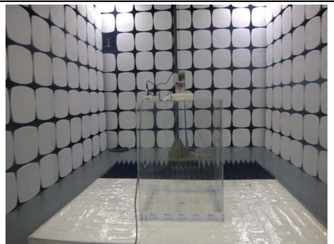
Radiated Spurious Emissions Test Setup Above 1GHz
