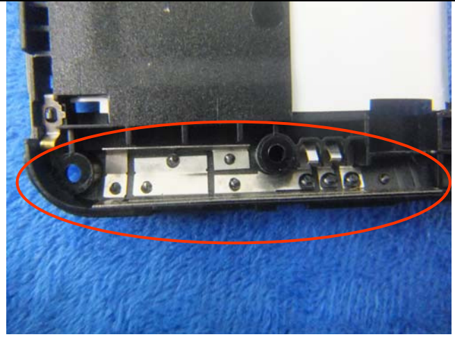
GSM/PCS/UMTS-FDD Antenna View
