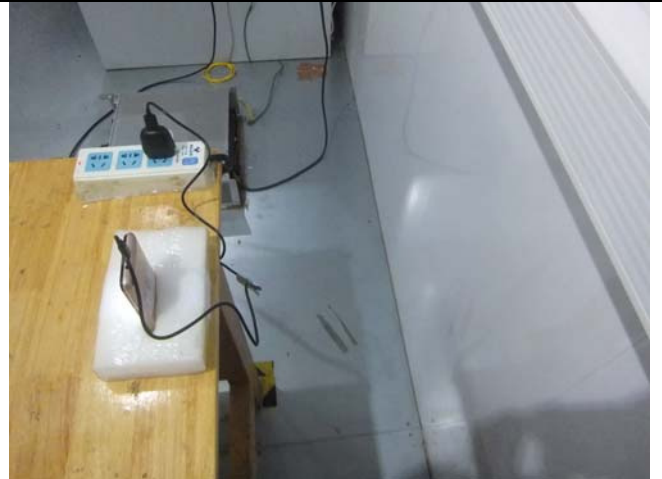
Conducted Emissions Test Setup Side View
