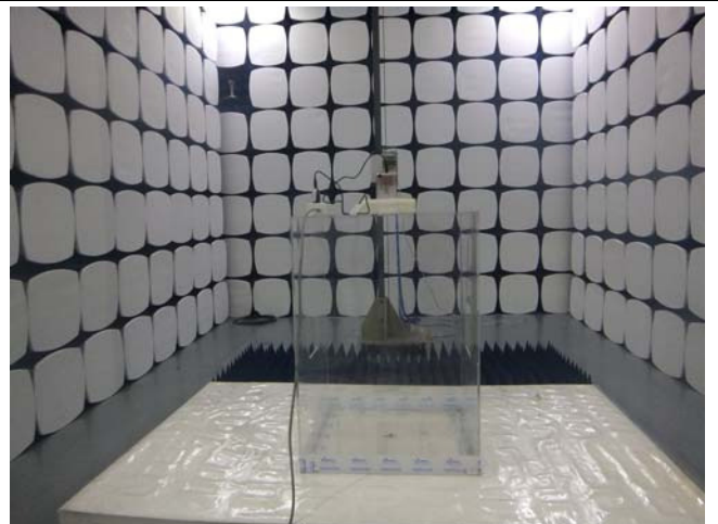
Radiated Spurious Emissions Test Setup Above 1GHz
