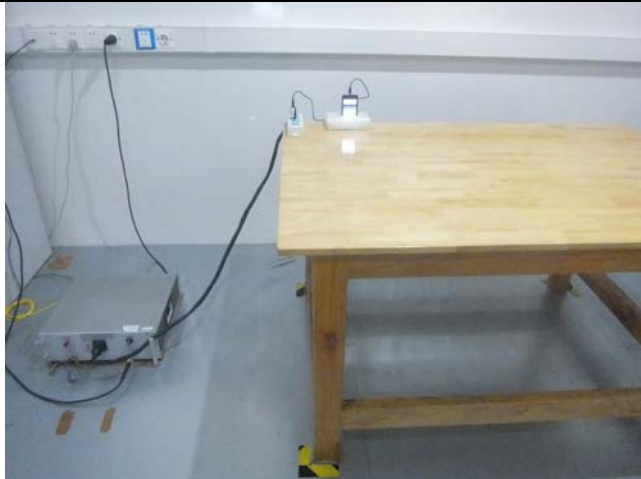
Conducted Emissions Test Setup Front View
