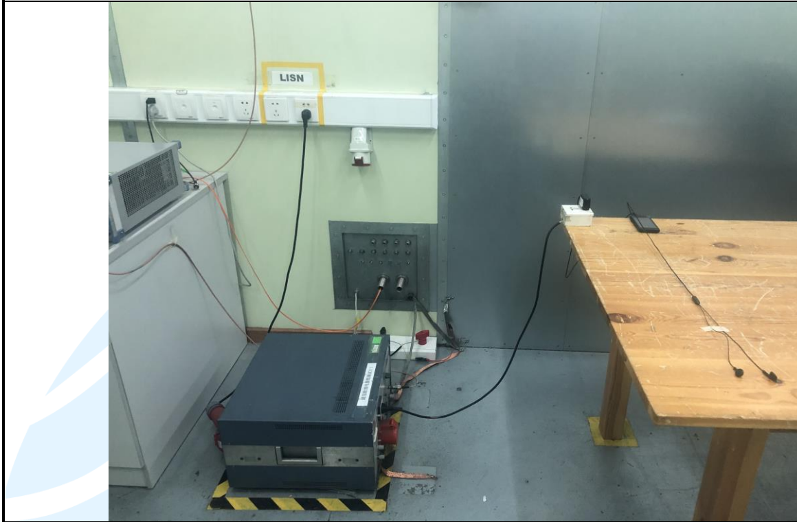
Conducted Emission Test Setup - Mode 4
