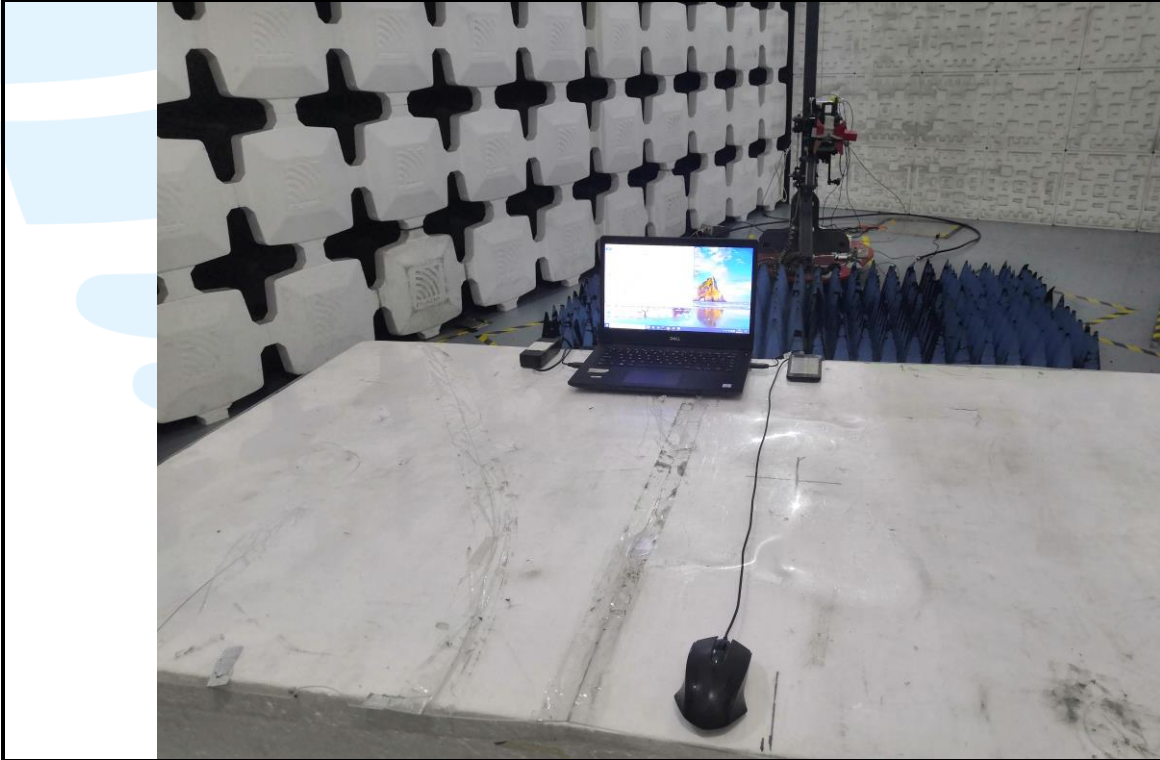
Radiated emission Test Setup (Above 1 GHz) - Mode 6
