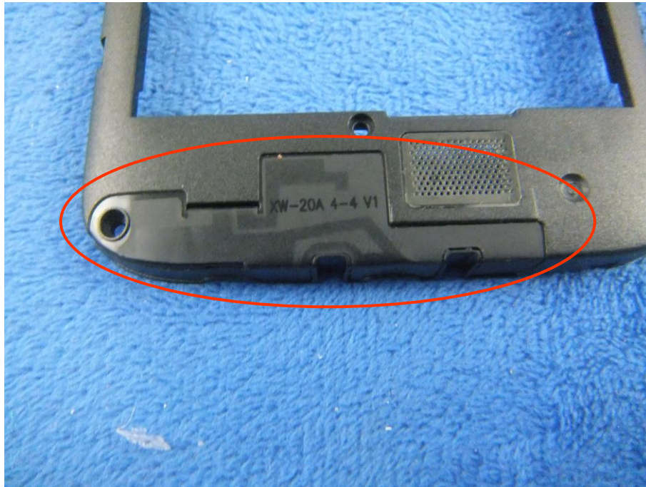
GSM/PCS/UMTS-FDD - Antenna View
