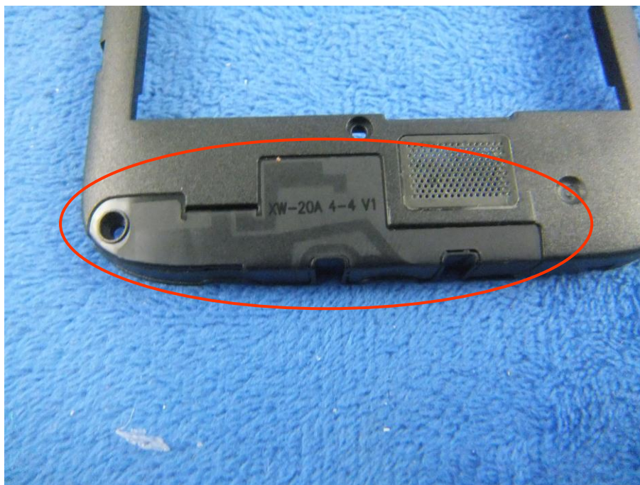
GSM/PCS/UMTS-FDD - Antenna View
