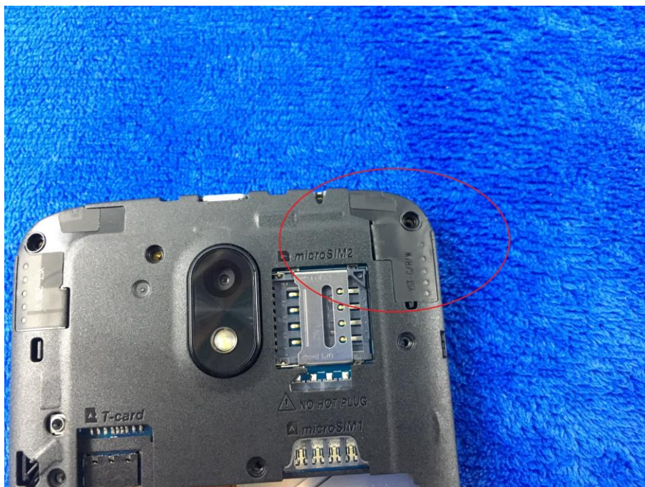
WIFI/BT/BLE/GPS - Antenna View
