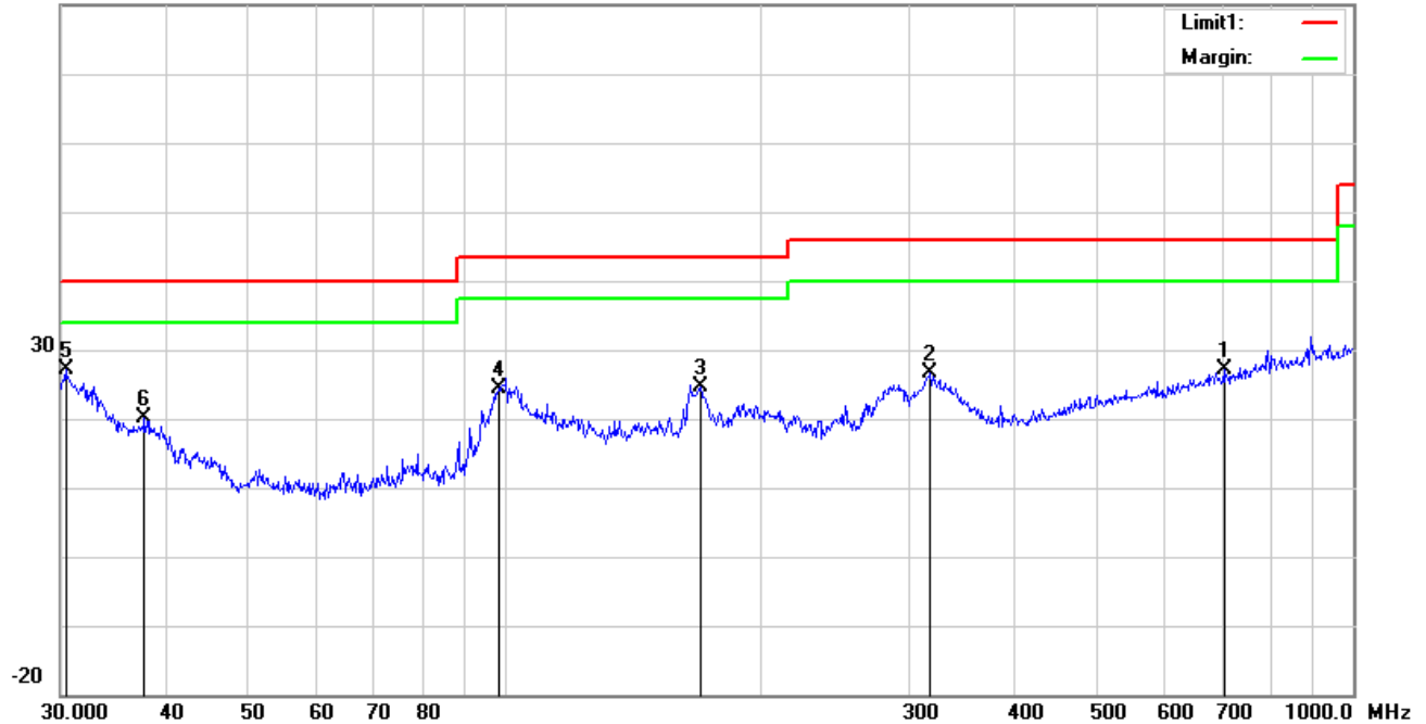
Horizontal Polarity Plot @3m
