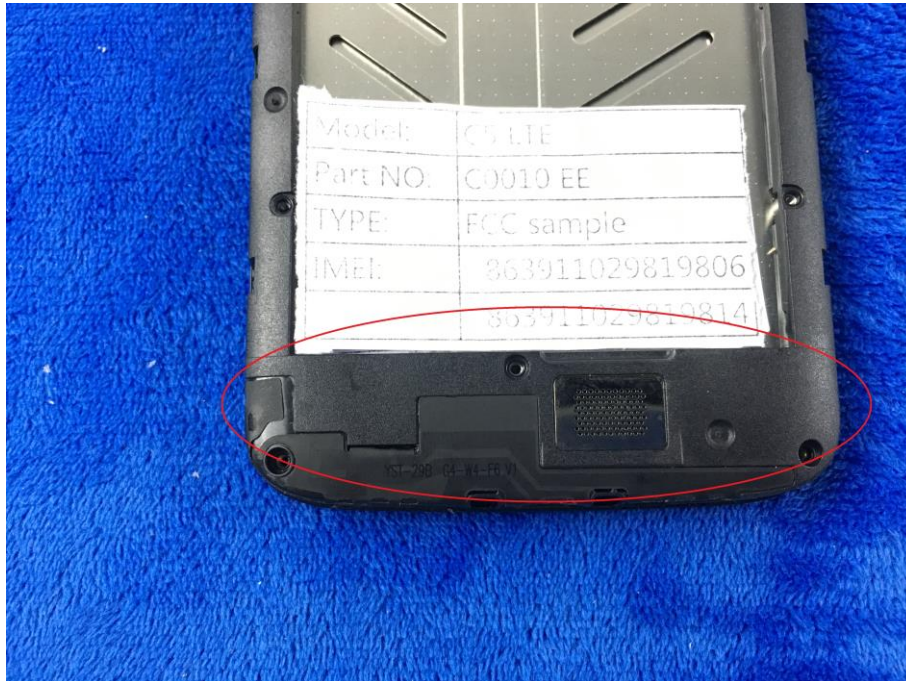
GSM/PCS/UMTS-FDD/LTE - Antenna View
