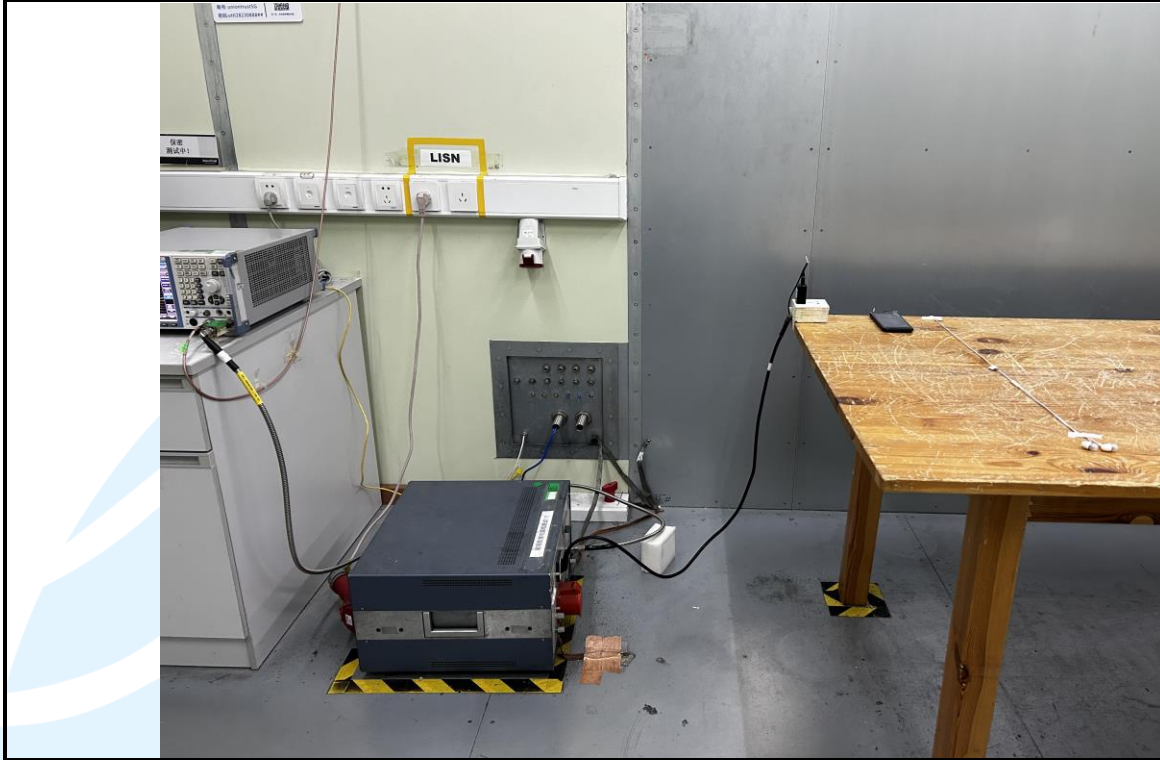
Conducted Emission Test Setup-3
