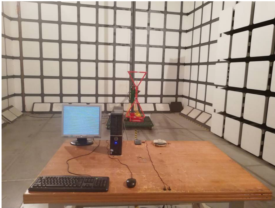
Radiated Emissions – Front View (Below 1 GHz)
