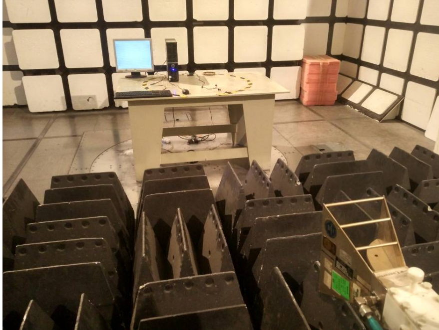
Radiated Emissions – Front View (Above 1 GHz)
