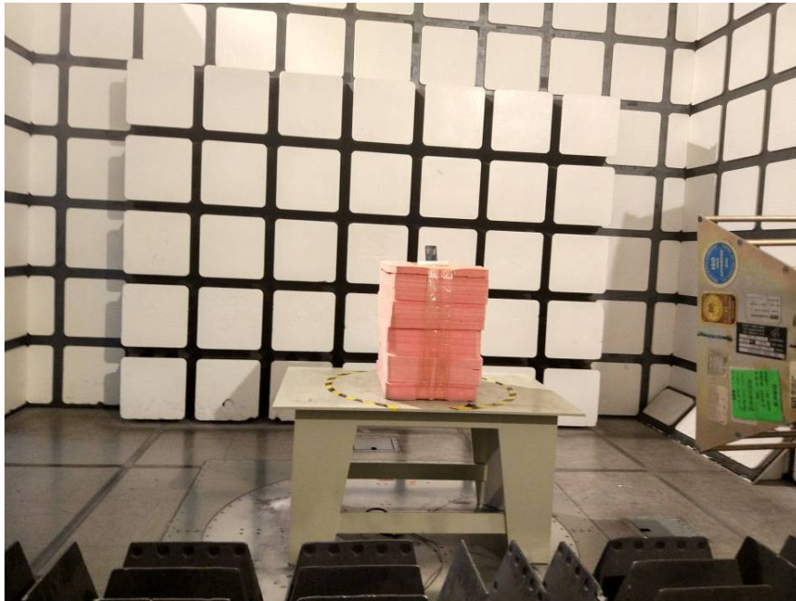
Radiated Emissions View (Above 1 GHz)
