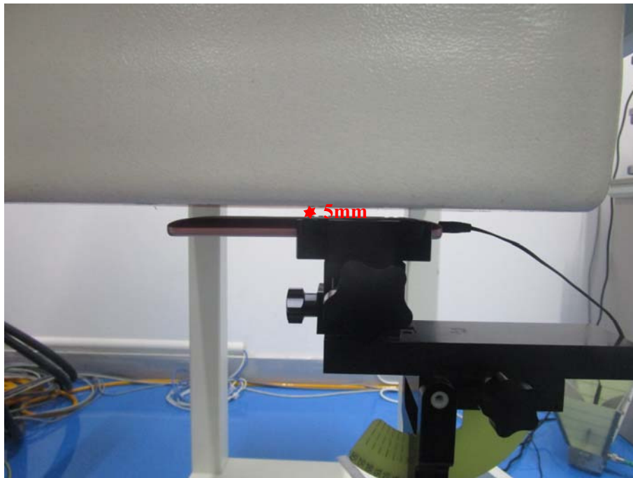
Body Worn Back with Headset Setup Photo(5mm)
