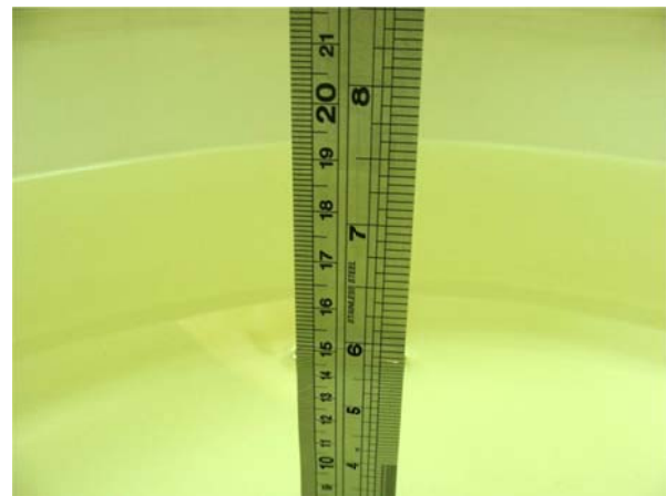
Fig 6.2 Photo of Liquid Height for Body SAR
