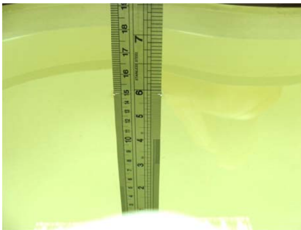
Fig 6.1 Photo of Liquid Height for Head SAR
