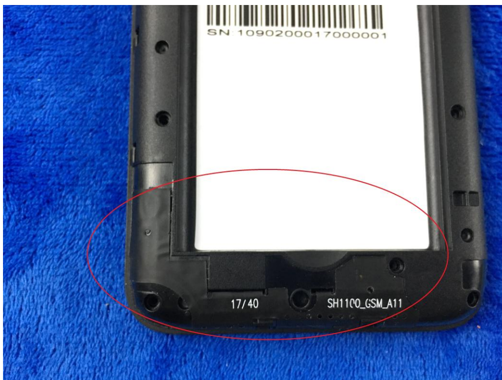
GSM/PCS/UMTS-FDD/LTE Antenna View
