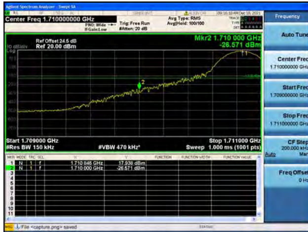
Band4 / 15MHz / High CH / QPSK / 1 RB
