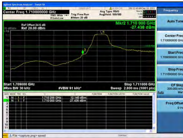
Band4 / 1.4MHz / High CH / QPSK / 1 RB
