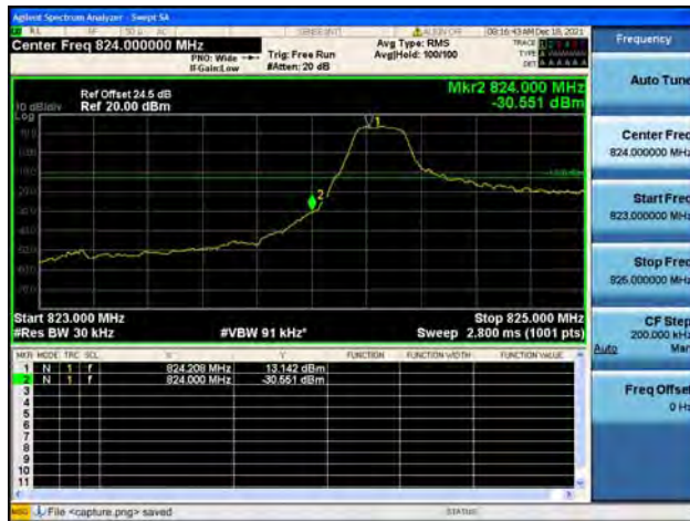
Band5 / 1.4MHz / High CH / QPSK / 1 RB
