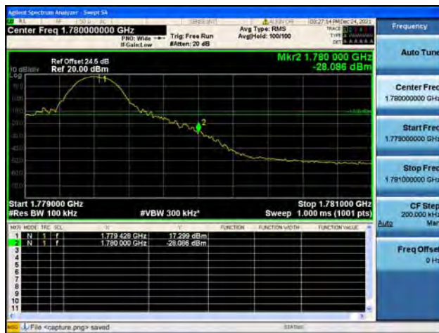
Band66 / 10MHz / High CH / QPSK / 1 RB
