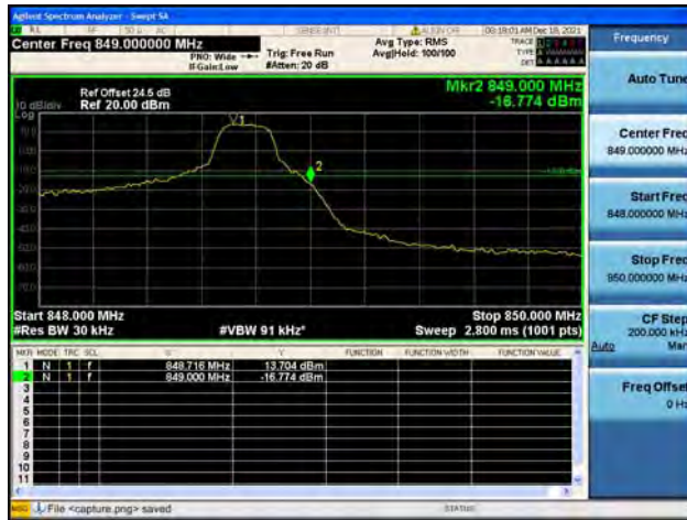
Band5 / 3MHz / High CH / QPSK / 1 RB
