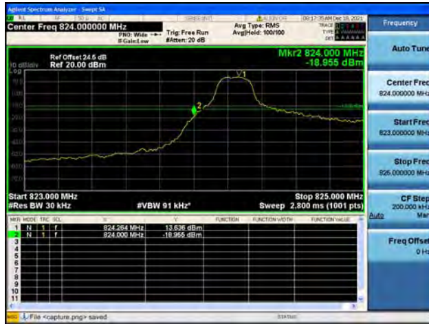
Band5 / 3MHz / High CH / QPSK / 1 RB
