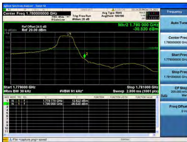
Band66 / 1.4MHz / High CH / QPSK / 1 RB
