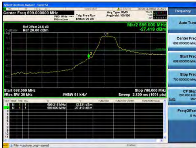
Band12 / 1.4MHz / High CH / QPSK / 1 RB
