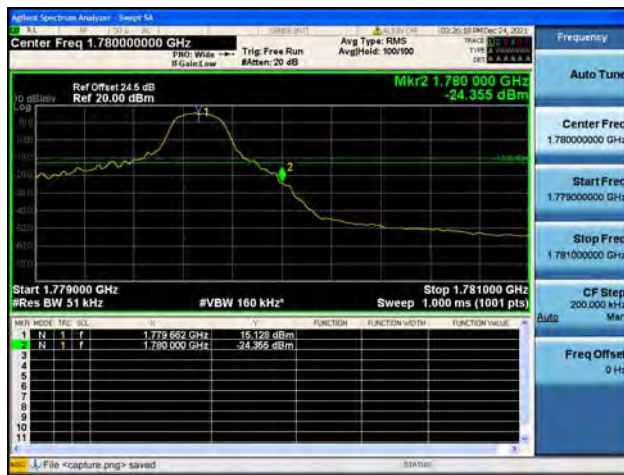
Band66 / 5MHz / High CH / QPSK / 1 RB
