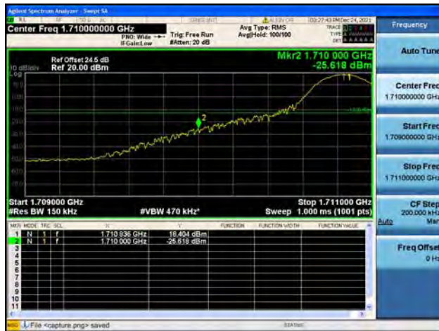
Band66 / 15MHz / High CH / QPSK / 1 RB
