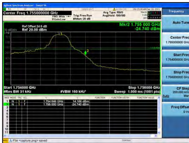
Band4 / 5MHz / High CH / QPSK / 1 RB
