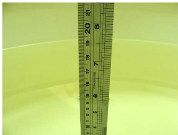
Fig 6.2 Photo of Liquid Height for Body SAR
