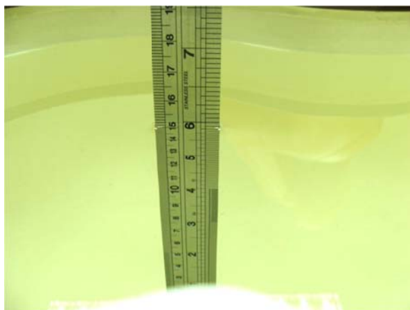
Fig 6.1 Photo of Liquid Height for Head SAR
