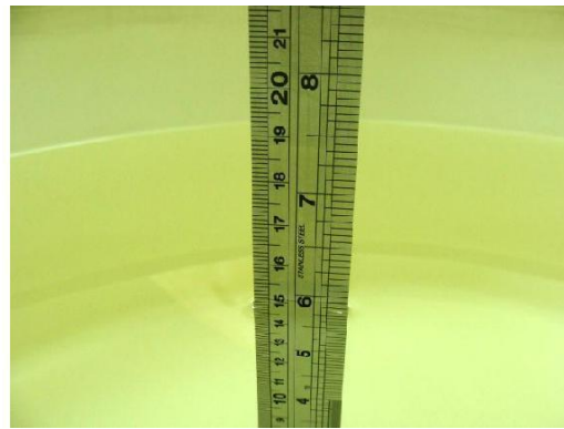
Fig 6.12 Photo of Liquid Height for Body SAR
