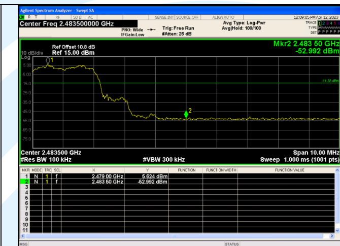
Out Of Band Emission(Right) 8DPSK_3-DH5_Channel Hopping
