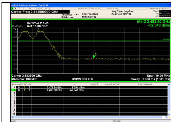
Out Of Band Emission(Right) GFSK_DH5_Channel Hopping
