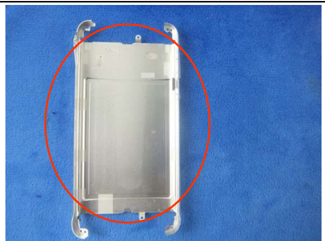
WIFI/BT/BLE/GPS – Metallic Antenna View
